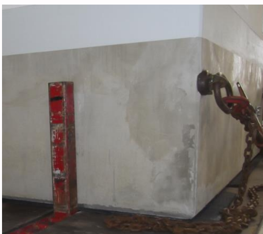
Fig. 16 Blocking with wedges or prisms
