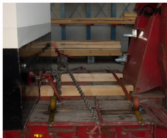
Fig. 16 Blocking with wedges or prisms
